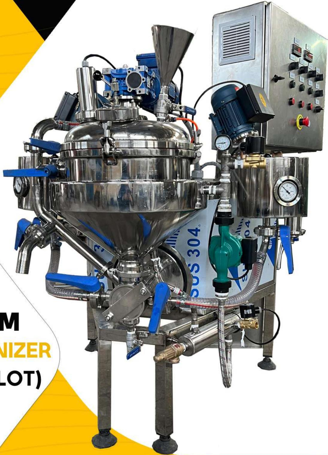
**Laboratory and pilot-scale vacuum homogenizer mixers** are designed for small-batch production and R&D. They reduce financial risks by allowing efficient testing of product formulations before scale-up. Typical uses include pharmaceutical emulsions, food sauces, and cosmetic lotions. These mixers can be manufactured in a range of capacities, from small-scale laboratory volumes up to 30 liters.
